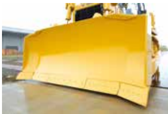
Semi-Universal blade (with hydraulic tilt)
